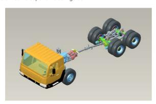
○ The combination of Fast 8-speed gearbox and single reduction axle features large speed ratio range and strong gradeability, which meets the requirements of low gradeability speed and high traveling speed.
